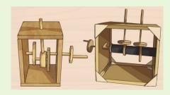
They first made a simple cam mechanism using a lolly sick and thick card. This meant they were able to clearly see the movement.
